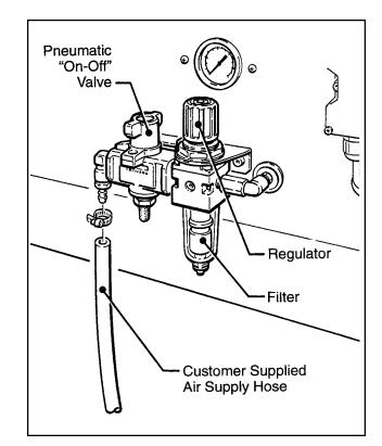
Figure 2-3 – Pneumatic Connection
